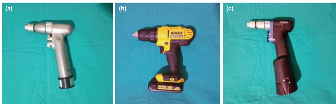
Fig. 1: Drills used in experiments: (a) Drill 1: Aesculap® Acculan 3. (b) Drill 2: Dewalt® (c) Drill-3: Synthes TRS Modular Drive®.
