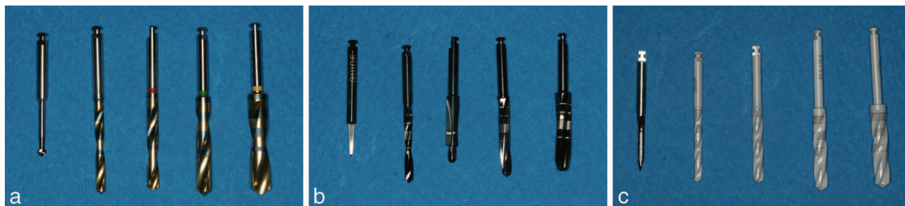
FIGURE 1. The implant drill systems. (a) The TiN-coated drill served as a control. The diameters for each drill sequence were 1.8, 2.0, 2.5, 3.2, and 4.2 mm (left to right). The color of the TiN coating was gold, as is typical. (b) The WC/C-coated drill had a black coating. The diameters were 1.5, 2.0, 3.0, 3.4, and 4.3 mm (left to right). Note that the third drill was not a twist drill but a pilot drill that enlarged a hole from 2.0 mm to 3.0 mm in diameter; the pilot drill was used as recommended by the manufacturer. (c) The zirconia ceramic drill was white in color. The diameters were 1.7, 2.0, 2.8, 3.5, and 4.2 mm (left to right).
